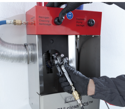
1. Flushing and cleaning of material passages and air cap (approx. 20 sec.)
