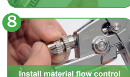
8 Install material flow control screw
