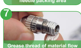
7 Grease thread of material flow control screw
