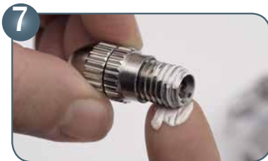
Grease thread of material flow control screw
