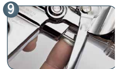
Grease visible part of air piston rod
